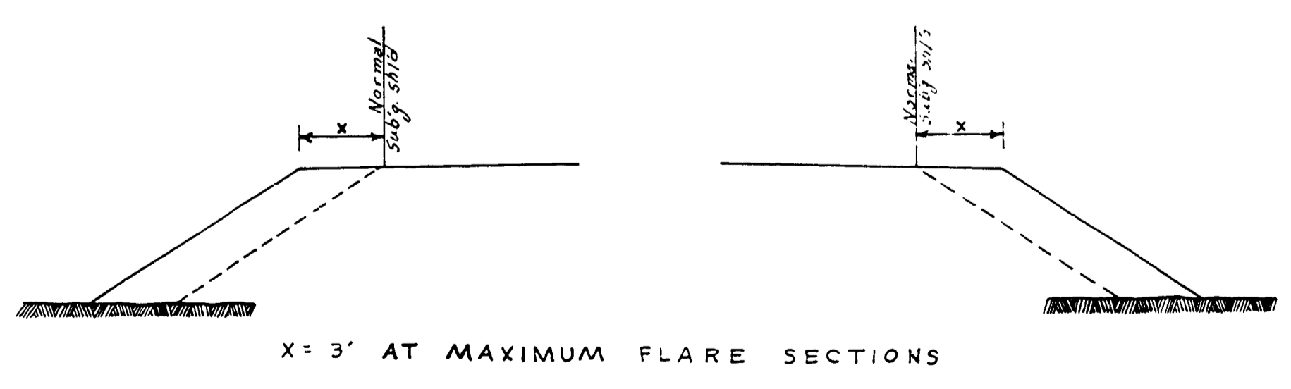
GUARD RAIL FLARE SECTIONS
